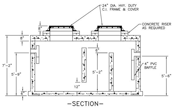
PRECAST CONCRETE 2000 GALLON COMMERCIAL GREASE INTERCEPTOR
